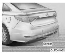
The Rear Parking Assist System assists the driver during reverse movement of the vehicle by chiming if any object is sensed within the distance of 50 inches (120 cm) behind the vehicle.
