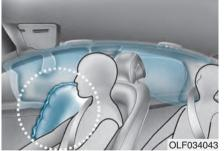
Your vehicle is equipped with a side air bag in each front seat. The purpose of the air bag is to provide the vehicle's driver and the front passenger with additional protection than that offered by the seat belt alone. The side air bags are designed to deploy only during certain side impact collisions, depending on the crash severity, angle, speed and point of impact.
