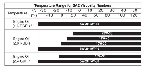
\*1 For better fuel economy, it is recommended to use the engine oil of a viscosity grade 5W-30 (API SM / ILSAC GF-4 / ACEA A5 or above). However, if the engine oil is not available in your country, select the proper engine oil using the engine oil viscosity chart.
