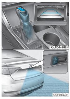
The Rear View Camera will activate when the engine is running and the shift lever is in the R (Reverse) position. This is a supplemental system that shows behind the vehicle through the navigation display while backing-up.
