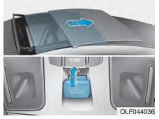
If you pull the sunroof control lever backward, the sunshade will slide all the way open then the sunroof glass will slide all the way open. To stop the sunroof movement at any point, pull or push the sunroof control lever momentarily.
