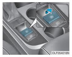
To apply the EPB (Electric Parking Brake):
