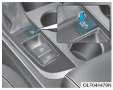
Push the button to turn off the Rear Parking Assist System. The indicator light on the button will turn on.
