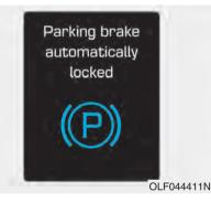
If the driver turns the engine off while Auto Hold is operating, EPB will be automatically applied. However, if you press the EPB switch within one second after the engine is turned off, the EPB will not be applied.
