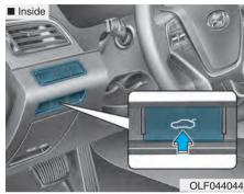
Use the trunk release button.3. Lift the trunk lid up.
