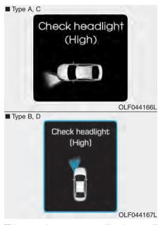
This warning message illuminates if there is a malfunction (burned-out bulb except LED lamp or circuit malfunction) with the headlamp. In this case, have your vehicle inspected by an authorized HYUNDAI dealer.
