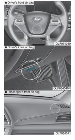
The purpose of the SRS is to provide the vehicle's driver and front passengers with additional protection than that offered by the seat belt system alone. The SRS uses sensors to gather information about the driver's and front passenger's seat belt usage and impact severity.
