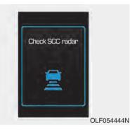
If the radar or cover is dirty or obscured with foreign matter such as snow, this message will appear. In this case, the system may not function temporarily, but it does not indicate a malfunction of the Smart Cruise Control System. Clean the radar or cover by using a soft cloth.
