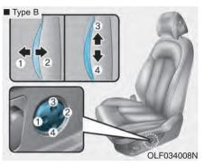
Lumbar support (for driver's seat, if equipped) The lumbar support can be adjusted
