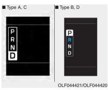
The pop-up displays the current gear position selected for 2 seconds (P/R/N/D).
