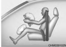
When the SRSCM detects a sufficiently severe impact to the front of the vehicle, it will automatically deploy the front air bags. Driver's front air bag (2)
