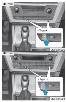
The air ventilation seats are provided to cool the front seats by blowing air through small vent holes on the surface of the seat cushions and seatbacks. When the operation of the air ventilation seats are not needed, keep the switches in the OFF position.
