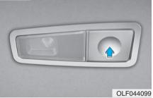
Rear Room Lamp  $\overline{xx}$ : Press this switch to turn the room lamp on and off.
