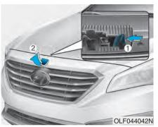
Raise the hood slightly, push the secondary latch up (1) inside of the hood center and lift the hood (2). After it has been raised about halfway, it will raise completely by itself.
