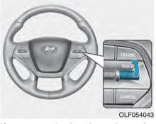
If any method other than the CRUISE lever was used to cancel cruising speed and the system is still activated, the cruising speed will automatically resume when you push the lever up (RES+) or down (SET-).
