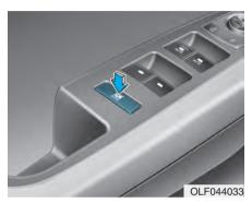
The driver can disable the power window switches on the rear passengers' doors by pressing the power window lock switch.
