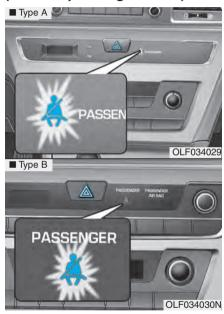
The front passenger's seat belt warning light will activate to the following table when the ignition switch is in "ON" position.
