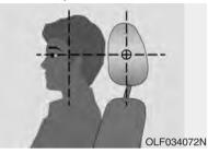
Adjust the head restraints so the middle of the head restraints is at the same height as the height of the top of the eyes.
