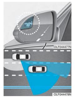
The Blind Zone Mirror (BZM) is a supplemental mirror that reduces the driver's blind zone by showing the rear side area of the vehicle. The blind zone mirror is equipped on the left-hand outside rearview mirror.
