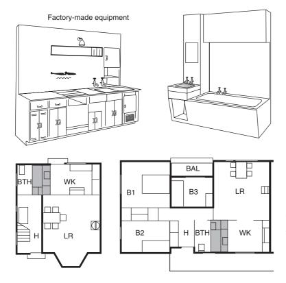
Figure 1.3 Post-war prefabricated housing: most contained the kitchen/ bathroom-combined unit made of pressed metal shown here in a threebedroom house and a three-bedroom flat (From Ministry of Health/Ministry of Works, Housing Manual 1944, HMSO, 1944, pp. 86 and 89).
