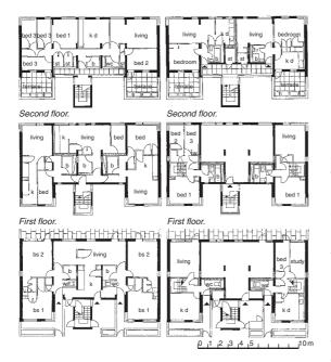
**Figure 2.13** PSSHAK, Adelaide Road. Sample plans: solid lines show the support structure; hatched areas show demountable party walls; open blocks show the "kit" (reproduced with approval from *AJ*, 21/5/75, p. 1073).
