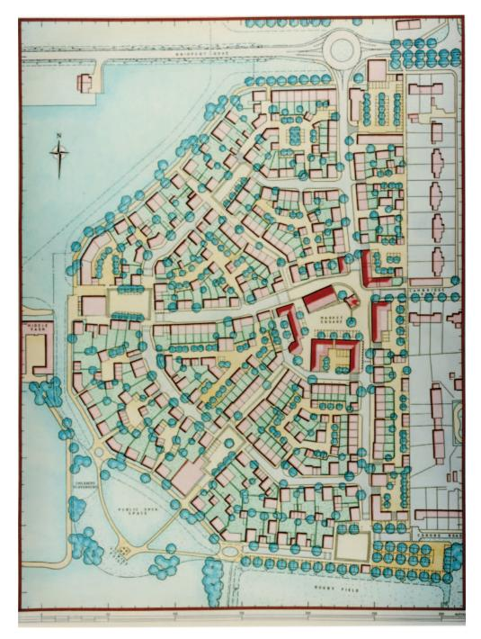
**Figure 3.126** Poundbury: layout of the first phase, laid out around a network of spaces into which vehicles have almost full access (plan by Alan Baxter & Associates and published in DETR, Places Streets and Movement. 1998, p. 30, Crown Copyright).
