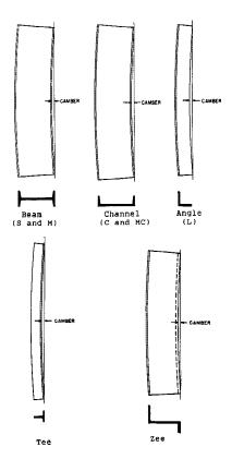
Positions for Measuring Camber of Shapes
