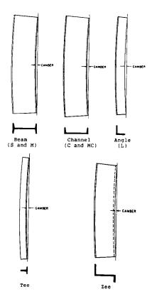
Positions for Measuring Camber of Shapes
